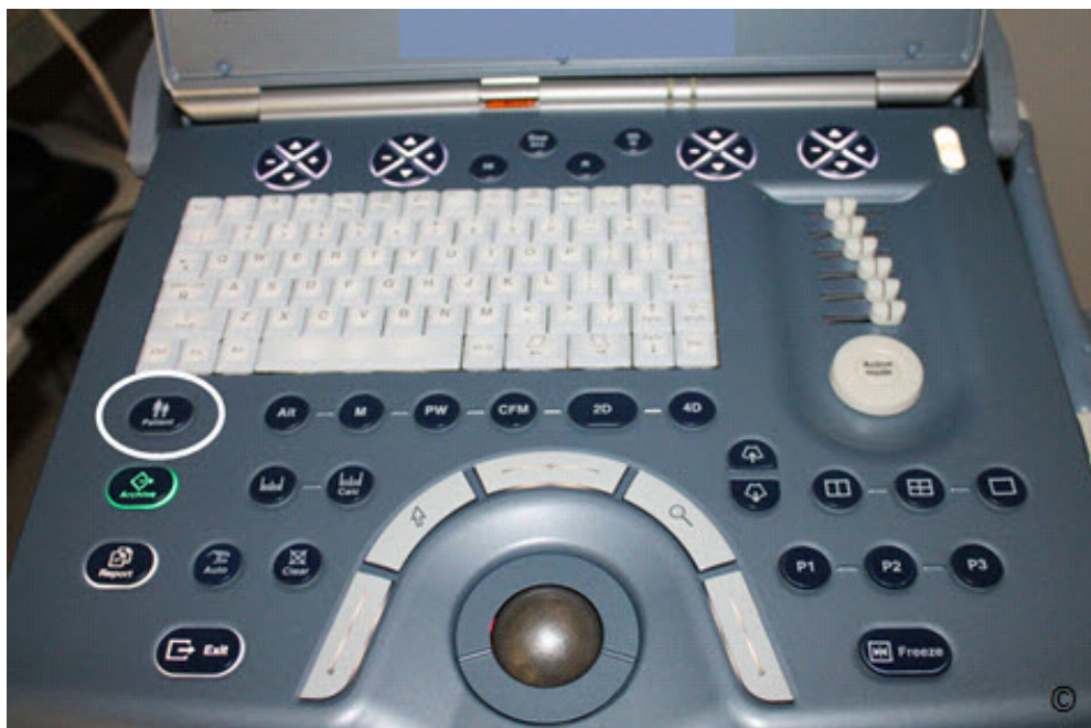
Figure 2.18: Consol of an Ultrasound equipment showing the knob identified as "Patient" (white circle), which leads you to a screen on the monitor (not shown) where patient identifiers are entered before initiating the ultrasound examination.
